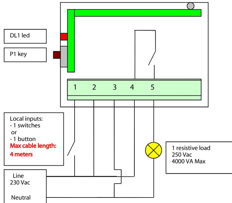
**Schematic 1.** Schematic indications for the control of one load
