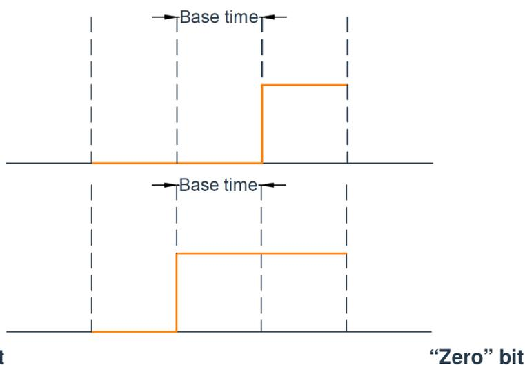
In case of fixed codes, the base time is measured during the learning process; the command is executed when a received frame has a base time within +/-10% of the measured value.
